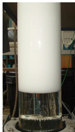
Figure -2 Stable bubble matrix formed, nearly uniform sized bubbles results in a distinct gas-liquid interface
